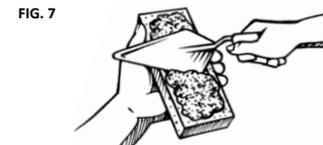
Note: In tight fit applications, before placing next unit, compact or remove the squeezed out mortar to allow adjoining unit to butt tightly. There shall be mortar between the units but the joint will be less than  $\frac{3}{8}$ ."
